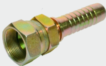
FITTING : MJF-ST (Komatsu) Metric Thread Female 74° Cone Seat Double Hexagon Fitting
